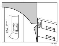
If the 2 tray finisher or the booklet finisher is attached to the printer, detach it before checking the earth leakage breaker.
