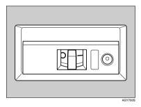
Move the earth leakage breaker to the "O" position.
