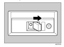
Reset the earth leakage breaker by moving it to the " | " position.
