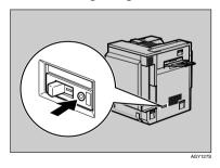
Make sure the earth leakage breaker is in the neutral position between "O" Off and " | " On.
